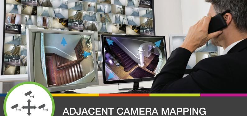
The CathexisVision Adjacent Camera Mapping Feature allows for simplified and accurate camera selection, streamlining the process to follow people or specific incidents taking place on site, by eliminating the need to remember camera names and locations in a crisis.
