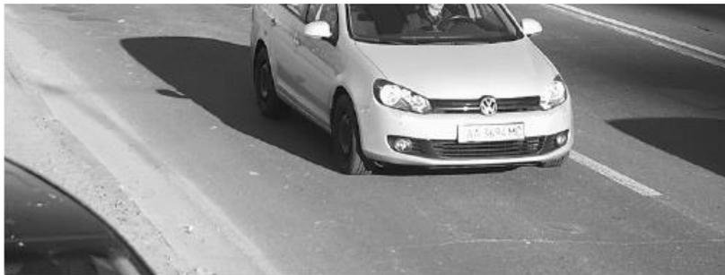
**Solution:** License plate is overexposed, image parameters should be adjusted. You can either adjust the shutter speed, or disable the IR-Led(for the night)
