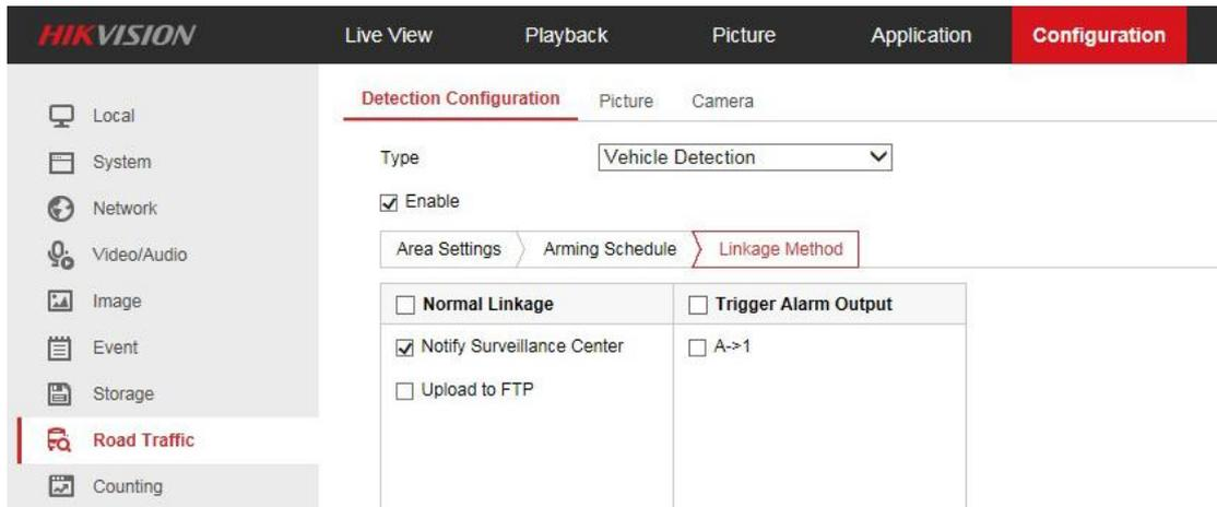
Fig.4 Linkage Method Configuration
