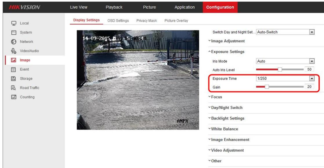
Fig.8 Recommended Exposure Time and Gain
