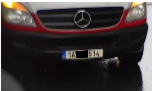
**Solution:** Reduce the exposure time to 1/250 or 1/500 depending on vehicle speed and lighting.
