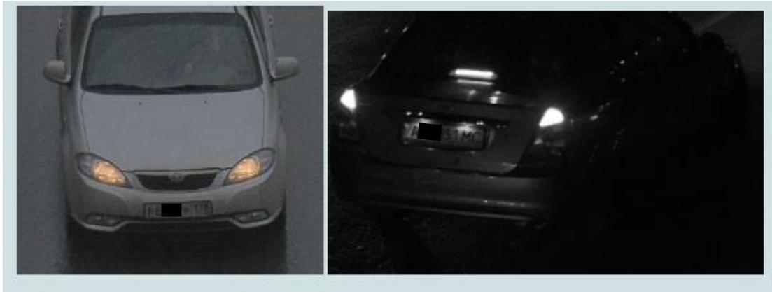
**Analysis:** Recognition performance is degraded with insufficient light. The camera must be set to night mode and infrared light should be used.
