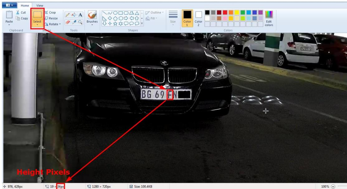
Fig.2 Measure the Plate Width
