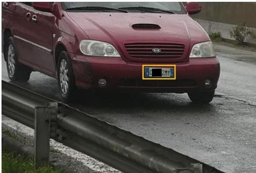
**Solution:** It seems that LP is well lit and readable by eye. However, if we measure full frame in photoshop, we will see that ANPR width is under 190px which is not enough. License plate width in the frame should be increased and be at least 90 pixels.
