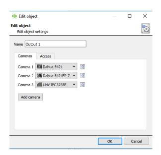
Adding a camera to an object will mean that, whenever there is an event on that object, the recording from that camera will be related to the time and date of the object event, in the Integration database.
