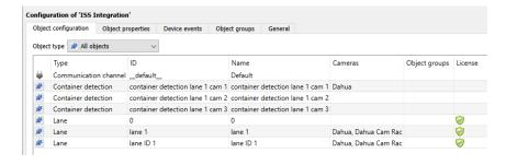
The object configuration tab is the tab where all the individual objects that comprise the integration may be viewed. The ISS integration device has four object types Container detection, Lane, and Communication channel.
