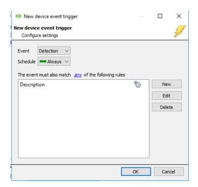
For example, within the any device event option, choose the type of device Event to be the trigger. Choose an event type from the drop-down menu.
