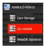
When the databases tab opens, select the relevant integration database from the database panel that opens on the left-hand side. The databases are ordered under the NVRs that they are attached to.
