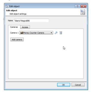
Adding a camera to an object will mean that, whenever there is an event on that object, the recording from that camera will be related to the time and date of the object event, in the Integration database.
