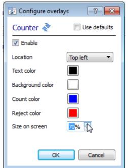
**Location** will define where on the camera feed's image the overlay is positioned.
