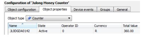
The Object properties tab allows you to view the objects, sorted by type. In the case of the Julong device you will have the options of viewing by **Counter.**
