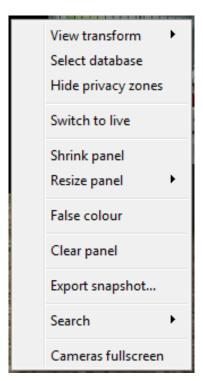
**View transform:** Allows transforming images for cameras with special lenses. (For example, 360-degree cameras.)
